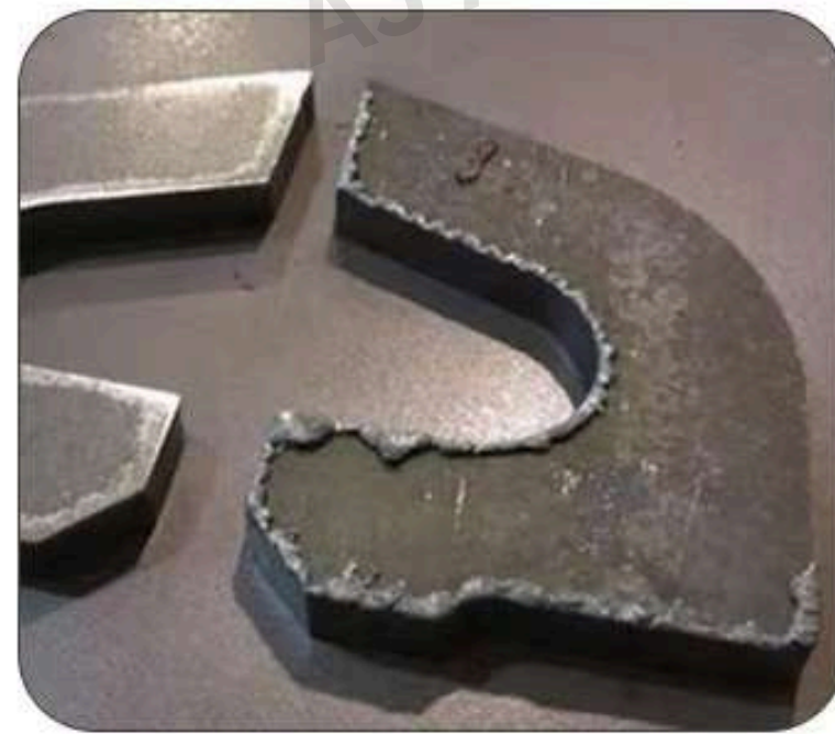
Burr removal from cut parts (deburring)
