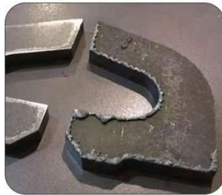
Burr removal from cut parts (deburring)
