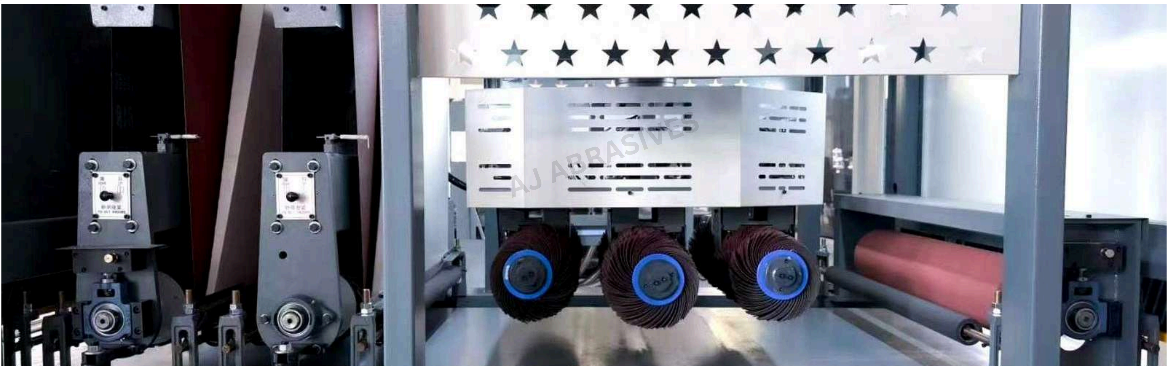
DUAL ABRASIVE BELTS + 1 ROTATING ROLLER + 1 POLISHING ROLLER
